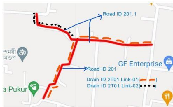
Figure2: Road location(ID-201) along with proposed side Drains
